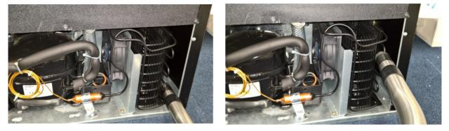
② Use vacuum nozzle to remove any debris
